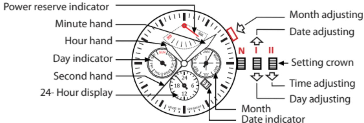
**DATE ADJUSTMENT:** Pull out the crown till position 1 and adjust the date by turning it counter-clockwise, then push the crown back into its neutral position [ N ].
